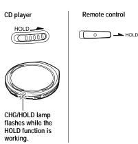
You can use the HOLD function with both the CD player and remote control. You can still operate your CD player using the remote control when HOLD on the remote control is set to off.
